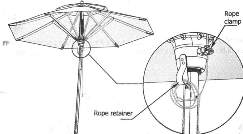
Once the umbrella is fully opened, lock the rope by pressing it into the rope clamp. up the loose rope, then place it in the leather rope retainer.
